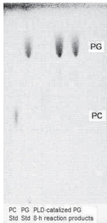
FIG. 1. TLC analysis of phospholipase D (PLD)-catalyzed transphosphatidylation of PC into phosphatidylglycerol (PG). Std, standard.
